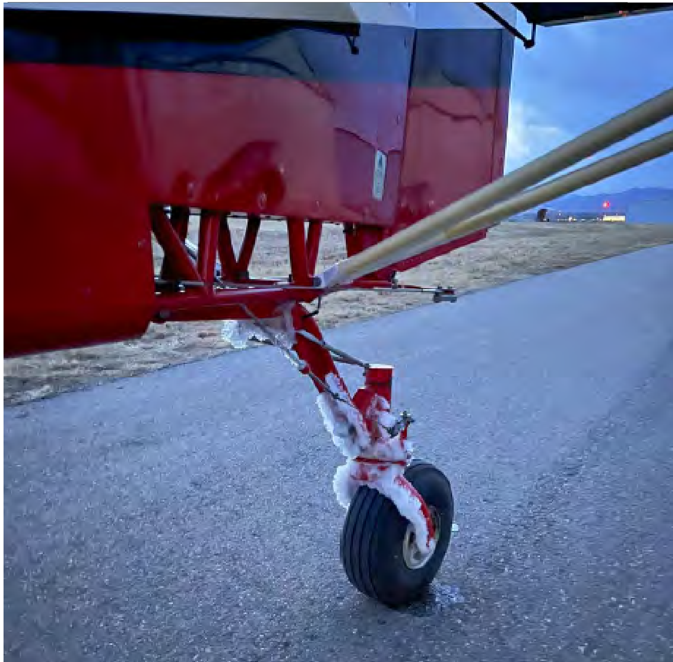
Ice on the landing gear of Air Tanker 861 after dropping water on the Oak Fire, Dec. 27, 2021. Photo by Chief Pilot Chris Doyle.
